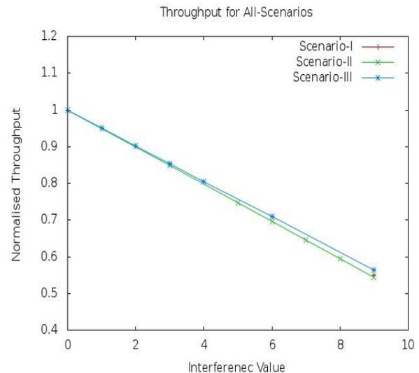
Fig.2 Normalised Throughput vs. Interference value
