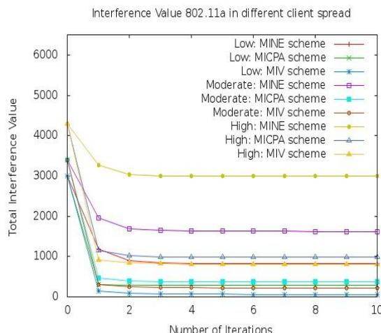
Fig.5 Total interference value for all three schemes for different client spread
