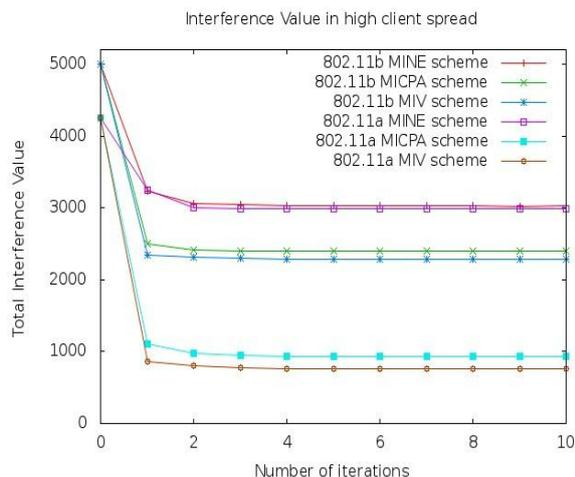
Fig.4 Total interference value for all three schemes for high client spread
